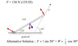
(ii) The vertical component of *R*:  $W - F \sin 60^\circ = 39.24$  N (upwards) The horizontal component of *R*:  $F \cos 60^\circ = 67.97$  N (leftwards) The magnitude of *R*:  $\sqrt{39.24^2 + 67.97^2} = 78.5$  N (78.484) The direction of *R*:  $tan^{-1}\frac{39.24}{67.97} = 30.0^\circ$  from the ground (29.998)
