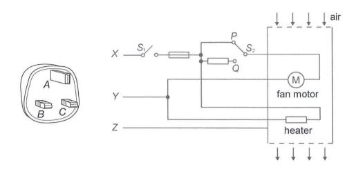
(a) Which pins (A, B and C) should wires X, Y and Z of the hand-dryer be connected to? (2 marks)
