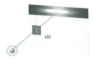
When a beam of monochromatic light of wavelength 650 nm passes through a narrow vertical slit, a bright fringe is formed on a screen as shown above. The fringe is about the same height as the slit, but it is much wider than the slit.
