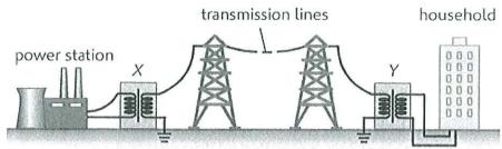
After passing through the transmission lines, the 50 kV voltage is stepped down to 220 V by transformer Y before it is delivered to the household user. The total current drawn by the house is 50 A. The efficiency of both transformers is 95%.
