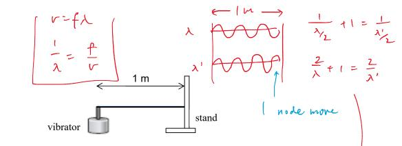
An elastic string stretched to 1 m long is fixed with one end to a vibrator and the other to a stand as shown in the figure. Stationary wave patterns are produced when the vibrator vibrates at 12 Hz and 16 Hz. No stable pattern is produced at frequencies between these two. Find the speed of the wave along the string.
