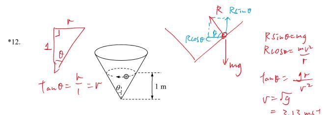
In the figure, a small sphere steadily describes a horizontal circular path in an inverted  $\frac{1}{\sqrt{2}}$ cone at a height of 1 m from the vertex. Find the speed of the sphere.
