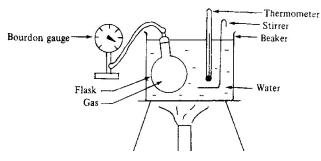
The above apparatus is used to study the relation between the temperature and the pressure of a fixed mass of gas at constant volume. Which of the following is NOT a precaution of the experiment? A unknown volume
