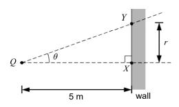
If the illuminance on the wall at X is E, what is the illuminance on the wall at Y which is at a distance r from X?
